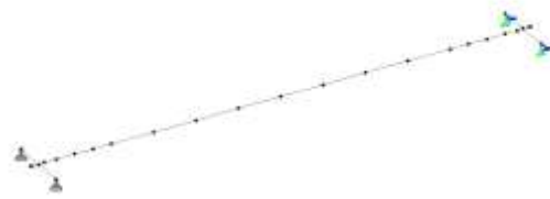
Fig 2: Grillage Model and Line beam model of PSC I Girder and Box girder
